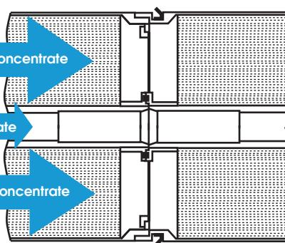
**Figure 6:** Comparison of cross-sections through the connection interface between two elements.(a) Standard sliding coupler, (b) Interlocking endcaps
