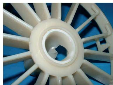
**Figure 16:** Rotta del tubo permeato nell' area adiacente alla connessione col tappo/ High-pressure failure of product water tube in area adjacent to weld with endcap.
