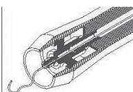
Rotate valve disk and push tubing until it reaches the end of the vessel.
