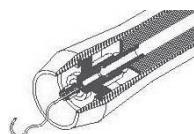
Insert 1/4" tubing into SamplePro valve until captured by first seal.
