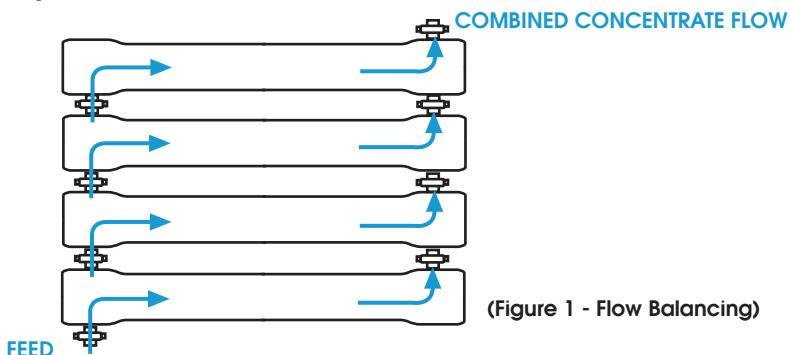
The down side of this arrangement is that it will cause the average feed flow pressure between the first and last vessel to be the at a maximum value, thus affecting permeate flow in the last vessel..
