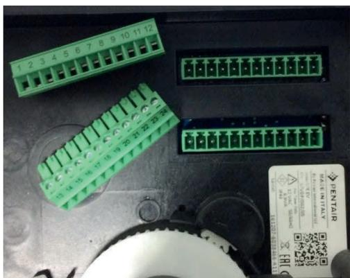
Morsettiere numerate con terminali a vite estraibili per connessione/ Numbered terminal blocks with removable screw terminals for connection
