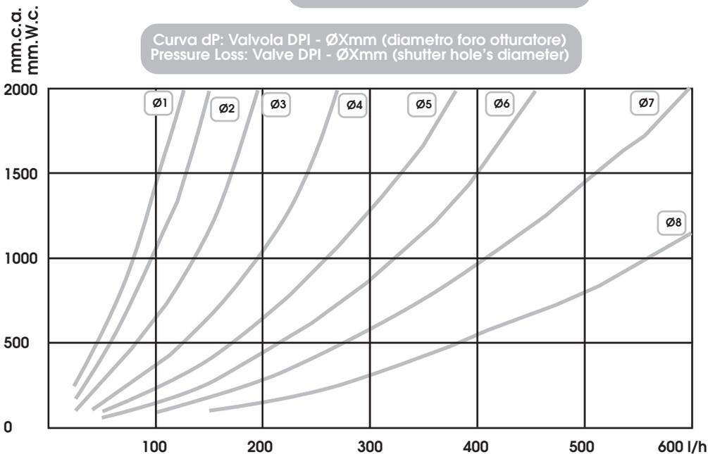
VALVOLA DOPPIA PORTATA PER PIASTRA SUPERIORE / DOUBLE FLOW VALVE FOR UPPER PLATE
