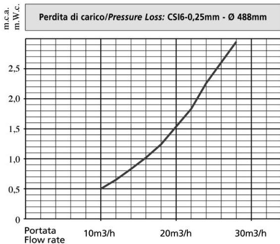
COLLETORE A 6 VIE INCLINATE - Attacco superiore 2" G / 6 TILTING WAYS COLLECTOR - Upper thread 2" G
