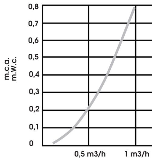
UGELLI A FESSURE VERTICALI MODELLO P7 / FILTER NOZZLES WITH VERTICAL SLOTS P7 MODEL
