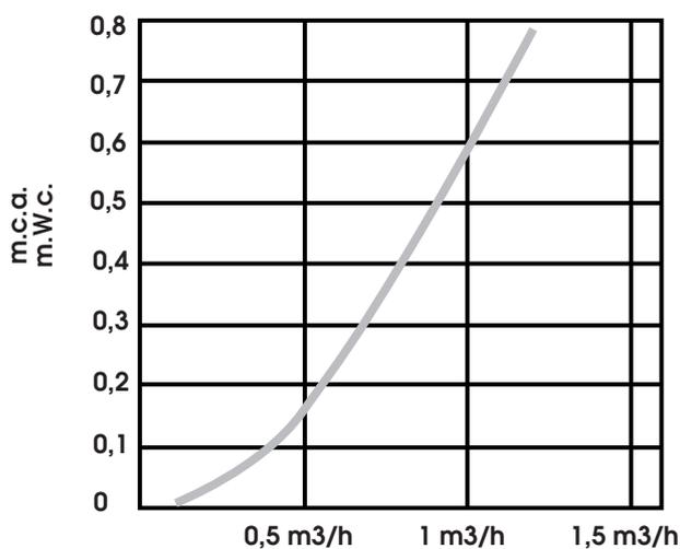
UGELLI A FESSURE VERTICALI MODELLO P6 / FILTER NOZZLES WITH VERTICAL SLOTS P6 MODEL
