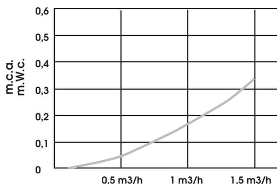
**UGELLI A FESSURE ORIZZONTALI MODELLO D/4.15 - FILTER NOZZLES WITH HORIZONTAL SLOTS D/4.15 MODEL**
