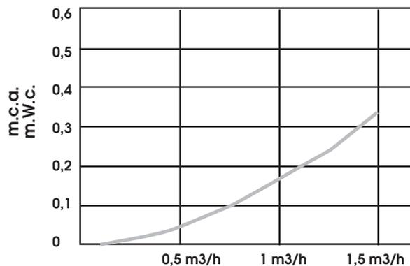
UGELLI A FESSURE ORIZZONTALI MODELLO D3 - FILTER NOZZLES WITH HORIZONTAL SLOTS D3 MODEL
