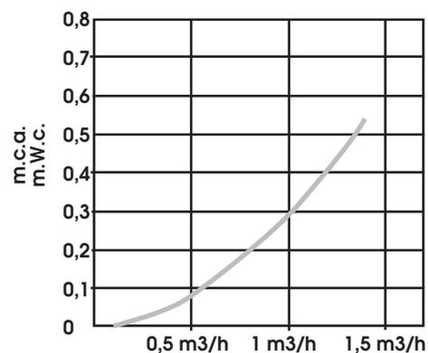
UGELLI A FESSURE VERTICALI MODELLO P5 / FILTER NOZZLES WITH VERTICAL SLOTS P5 MODEL
