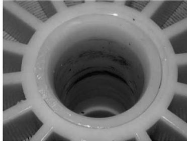
**Figure 3:** Evidence of o-ring wear inside a product water tube due to insufficient lubrication of the sliding seal.
